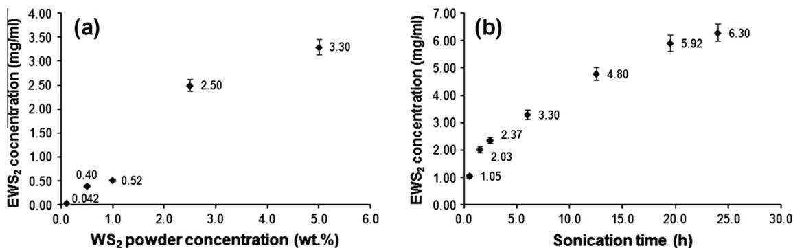
Fig. 1. EWS<sub>2</sub> concentration as a function of initial WS<sub>2</sub> powder concentration (a) and sonication time (b).
