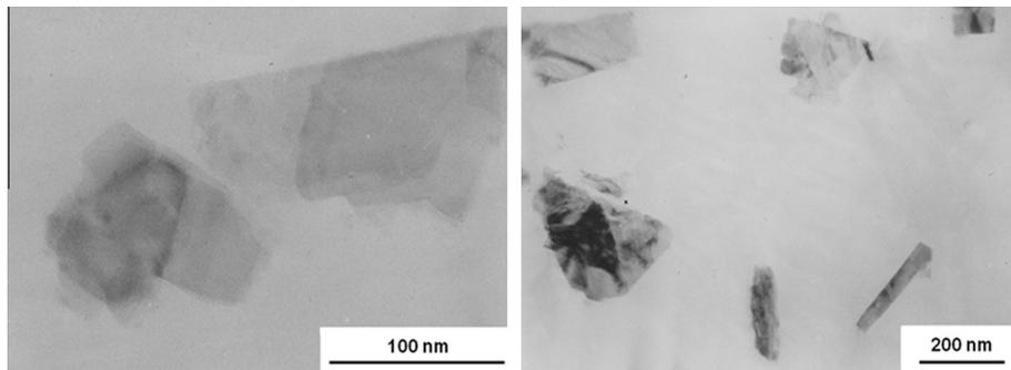
Fig. 3. TEM micrographs of EWS<sub>2</sub> dispersed in TEGDA.
