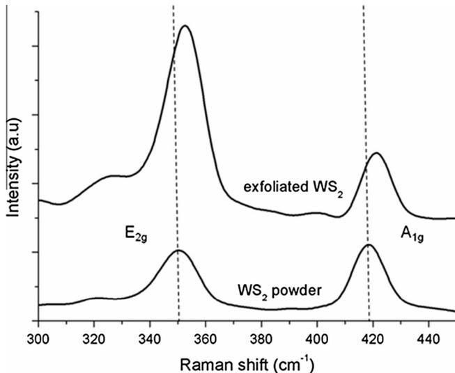
Fig. 4. Raman spectrum of EWS<sub>2</sub> compared with the spectrum of the pristine WS<sub>2</sub> powder.
