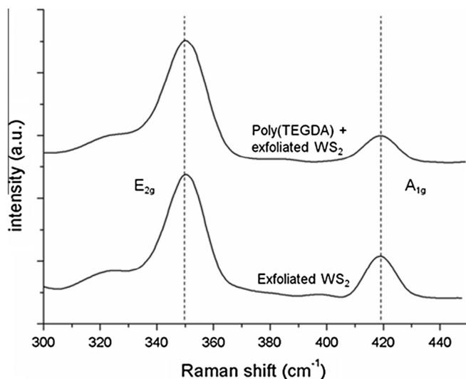
Fig. 6. Comparison between Raman signals of EWS<sub>2</sub> dispersed in the poly(TEGDA) matrix and EWS<sub>2</sub> deposited on PVDF filter.
