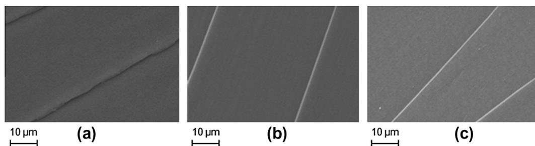
Fig. 7. SEM micrographs of poly(TEGDA) nanocomposites: neat polymer (a, sample B0) and polymers with 0.048 wt.% (b, sample B3) and 0.57 wt.% (c, sample B6) EWS<sub>2</sub>.
