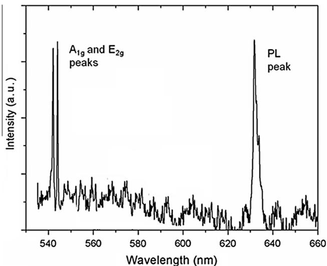
Fig. 5. PL peak for EWS<sub>2</sub> deposited on a PVDF filter.
