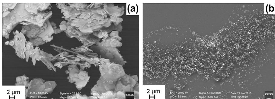
Fig. 2. SEM micrographs of pristine WS<sub>2</sub> powder (a), and EWS<sub>2</sub> deposited on a silicon substrate (b).
