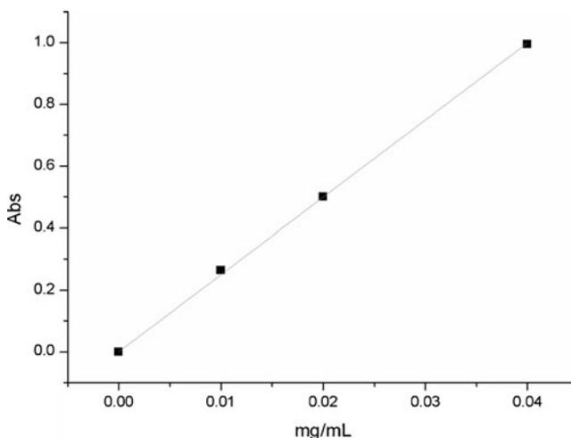
**Fig. 1** Optical absorbance (660 nm) as a function of graphene concentration in DMF. The Lambert–Beer behavior is exhibited, with an absorption coefficient of  $2,498 \text{ mL mg}^{-1} \text{ m}^{-1}$
