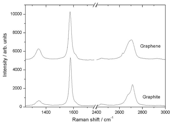
**Fig. 2** Raman spectra of graphene obtained from DMF dispersion (*top line*) and graphite (*bottom line*)
