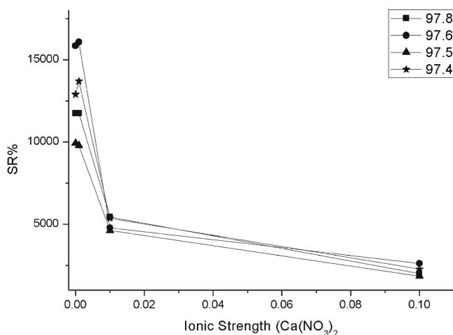
**Fig. 5** SR% as a function of ionic strength for different graphene amounts (Ca(NO<sub>3</sub>)<sub>2</sub> solution, sample 97.8=0 wt% of graphene, sample 97.6=0.01 wt% of graphene, sample 97.5=0.02 wt% of graphene, sample 97.4=0.06 wt% of graphene)
