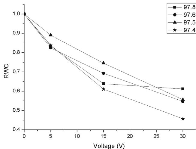
**Fig. 6** RWC of hydrogels as a function of the voltage applied for different graphene amounts (sample 97.8=0 wt% of graphene, sample 97.6=0.01 wt% of graphene, sample 97.5=0.02 wt% of graphene, sample 97.4=0.06 wt% of graphene)
