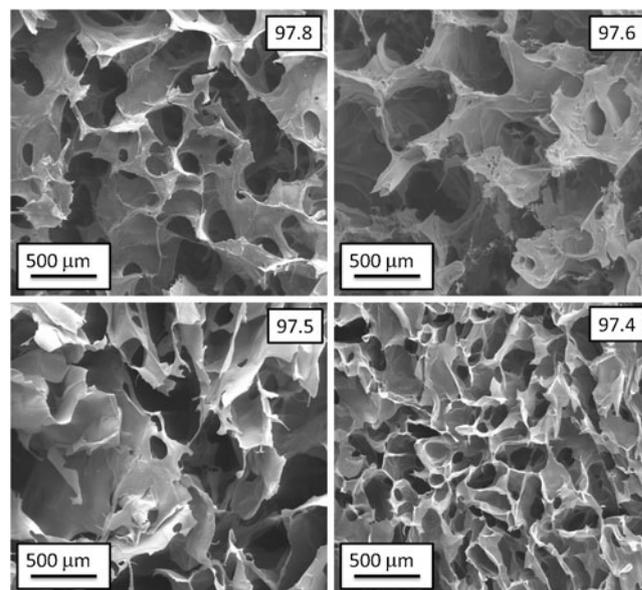
**Fig. 7** Micrographs of hydrogel samples (sample 97.8=0 wt% of graphene, sample 97.6=0.01 wt% of graphene, sample 97.5=0.02 wt% of graphene, sample 97.4=0.06 wt% of graphene)
