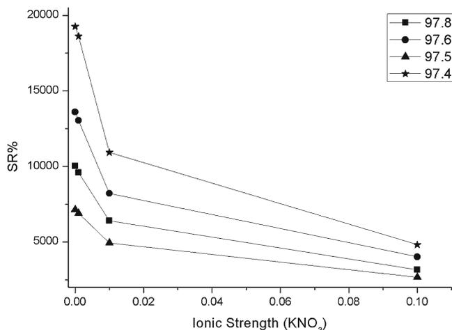
**Fig. 4** SR% as a function of ionic strength for different graphene amounts (KNO<sub>3</sub> solution, sample 97.8=0 wt% of graphene, sample 97.6=0.01 wt% of graphene, sample 97.5=0.02 wt% of graphene, sample 97.4=0.06 wt% of graphene)
