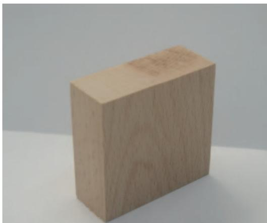
Fig. 2. – Photograph of one of the wood samples reported in this paper. All the samples have the same size. The dimensions are  $(5 \times 5 \times 2) \text{ cm}^3$ .
