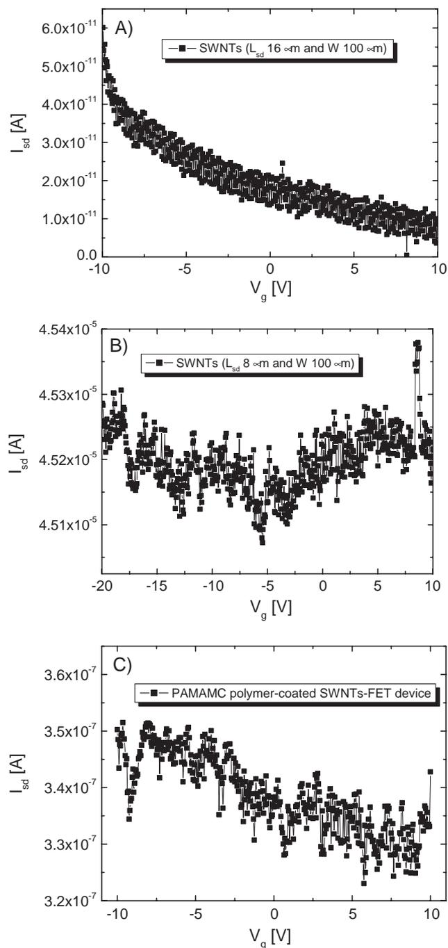
Fig. 3. A)  $I_{sd}$  vs  $V_g$  at  $V_d=0.5$  V for SWNTs-FET with a channel width of 100  $\mu\text{m}$  and a channel length of 16  $\mu\text{m}$ ; B)  $I_{sd}$  vs  $V_g$  at  $V_d=0.5$  V for SWNTs-FET with a channel width of 100  $\mu\text{m}$  and a channel length of 8  $\mu\text{m}$  C)  $I_{sd}$  vs  $V_g$  at  $V_d=0.5$  V for PAMAM/SWNTs-FET device with a channel width of 100  $\mu\text{m}$  and a channel length of 16  $\mu\text{m}$ .
