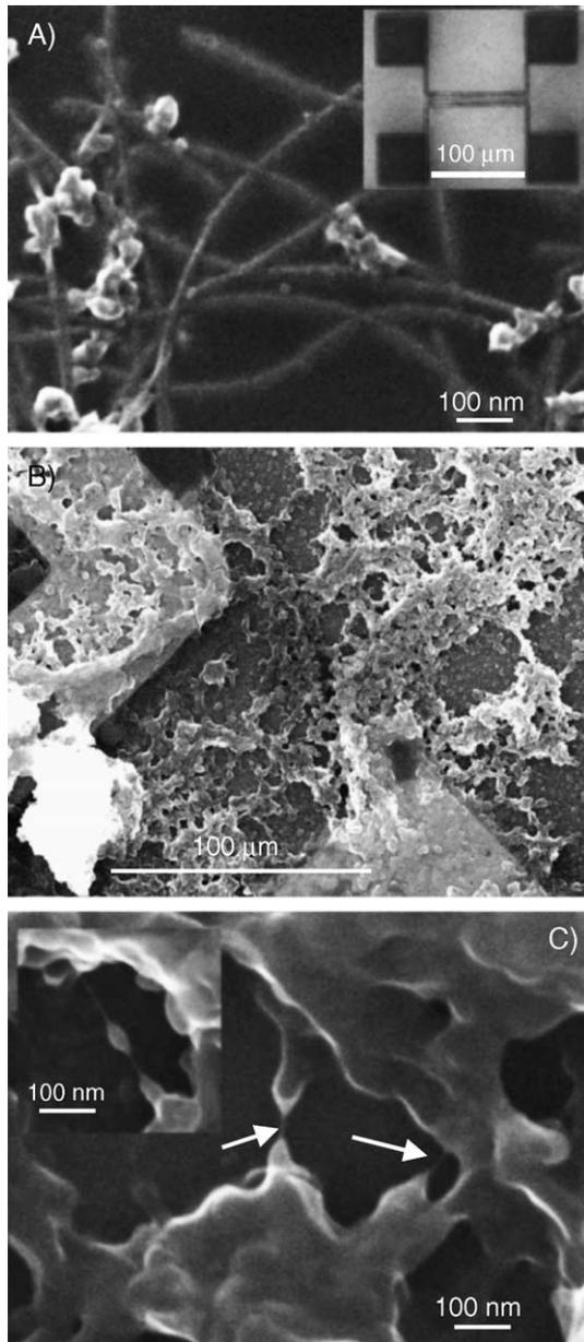
Fig. 1. SEM images of A) the specimen of pristine SWNT cross-linked bundles (the inset shows SEM micrograph of the device geometry), B) SWNTs dispersed in PAMAMC between the electrical contacts and C) SWNTs dispersed in PAMAMC (the arrows indicate the tubes; the inset shows SEM micrograph of PAMAMC coating SWNTs).
