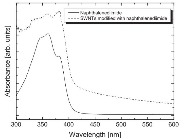
Fig. 2. UV–Vis spectra of naphthalenediimide and SWNTs dispersed in naphthalenediimide.
