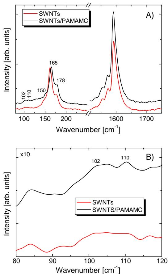
Fig. 4. A) Raman spectra of SWNTs and SWNTs modified with PAMAMC; B) Raman spectra of SWNTs and SWNTs modified with PAMAMC for wavenumbers below 120  $\text{cm}^{-1}$  with the signal multiplied by ten.
